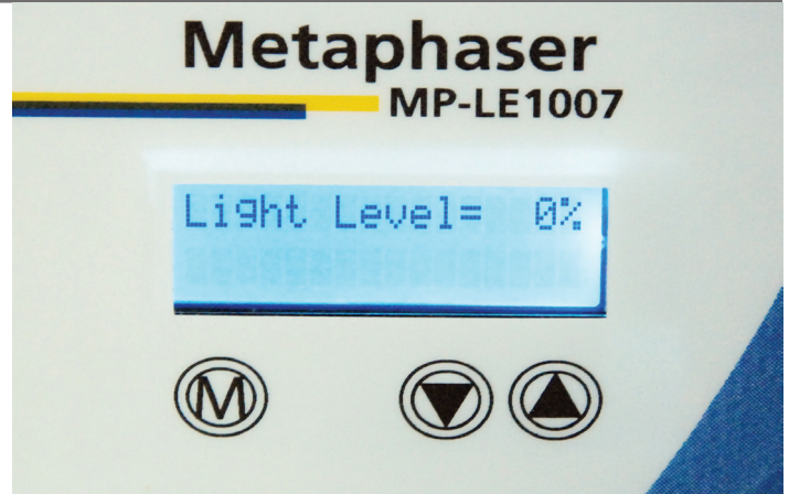
This image displays menu to change the intensity of the Metaphaser using the up and down arrows. (0% - 100%)
