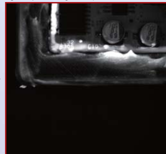
The High-output UV Light Unit has sufficient output for fluorescent observation.
